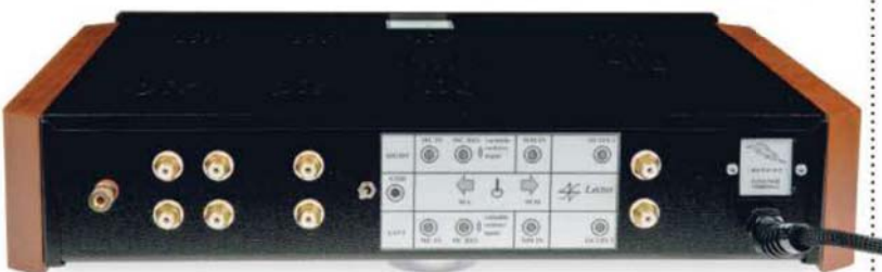
ABOVE: The extra pair of phono sockets is for plug-in resistors which adjust MC load impedance. When none are fitted, as here, the load is 47k ohms
